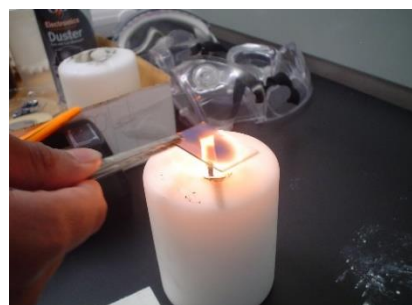
Figure 6 Applying Soot Layer
