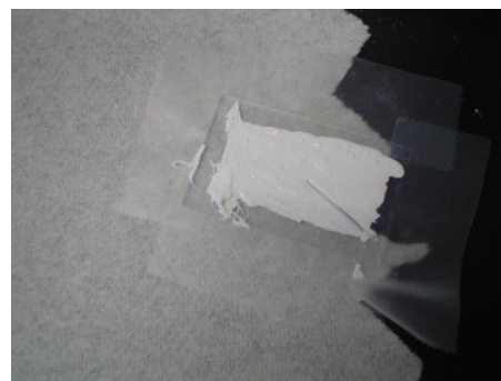
Figure 1 Conductive Glass with TiO 2 Paste Drying on It
